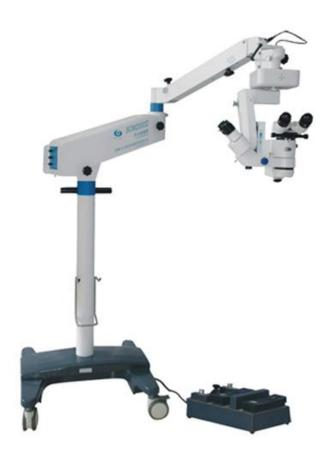
SOM2000D operation microscope is an advanced double binocular operation microscope designed for two men, ZOOM magnification and foot switch. ZOOM magnifications for main microscope, 4X~25X continuously adjustment.
